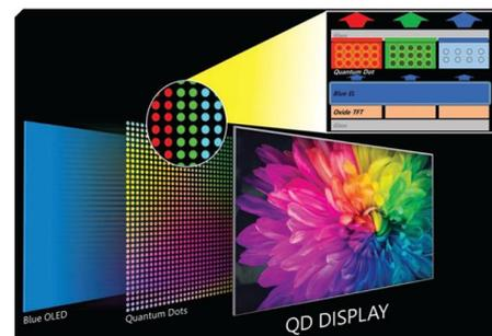
Figure 2. The structure of QD-OLED.
